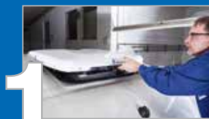
Remove roof hatch, insert unit
